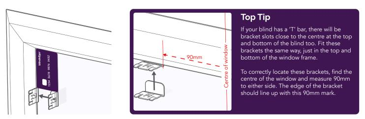
Locate the correct position for the side brackets by holding a credit card vertically in the corner of the glass - the bracket will sit in line with the edge of the card. Slide each bracket fully under the rubber seal.
