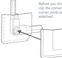
Before you slot the frames together, clip the corner cover pieces onto the corner joints so that they're firmly attached. Attach the side frames to the top and bottom by inserting the pegs on each corner section into their corresponding channels in the frames. Press the pegs firmly into place, the tension in the blind's cords will hold the frame together once fully assembled.
