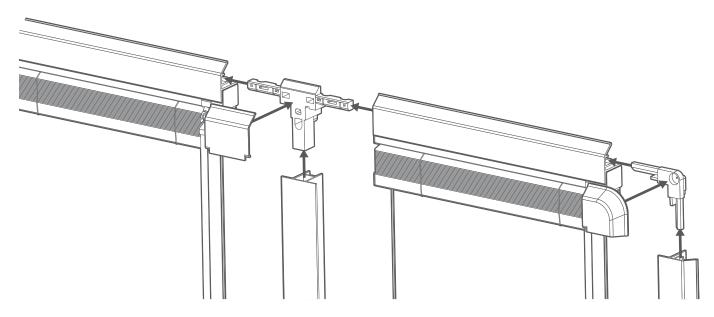
The top and bottom frames are connected to the side frames using the supplied corner pieces, then to the 'T' bar using the T-shaped connector pieces.
