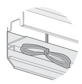
When you first unpack the blind, the cords will be tied to keep them together. Untie the knot to release the cords, so that you can spread out the blind ready for assembly.
