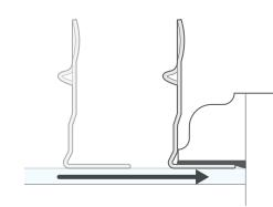
Locate the correct position for the brackets by holding a credit card or store card vertically in the corner of the glass - the bracket will sit in line with the edge of the card.
