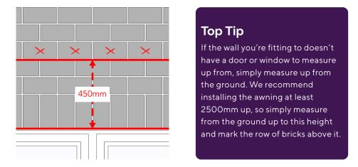
Using chalk or a pencil, mark the row of bricks at the top of the 450mm measurement. If 450mm falls on the mortar between two rows, mark the row above.
