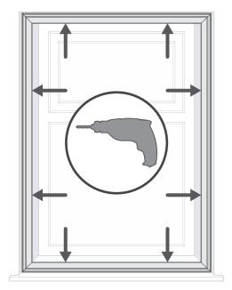
Making sure that the frame stays still and level, push the drill through each of the fixing holes you made in the frame and drill a small pilot hole in the surface you're fixing the shutter to (the inside of the recess). Now take your frame out of the window, you should be left with shallow pilot holes all around the recess - two for each side, the top and the sill.
