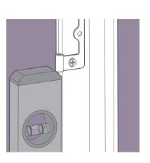
If you need to adjust the level of the frame then you can use the frame shims from your fitting kit. Fully insert the shim so that it is hidden by the frame.
