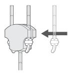
... Then slot the cords into the notches on the sides of the condenser, ensuring the knots at the ends of the cords are tight.
