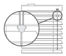
A breakaway cord condenser is pre-fitted to the lift cords so that when a horizontal force is applied to the cords entering the condenser, it safely releases the cords to eliminate any hazardous loops.
