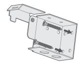
Where the brackets are screwed onto a facing surface (a wall or window frame)
