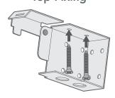
Where the brackets are screwed into the lintel (or 'ceiling' of the recess)
