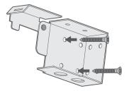
Where the brackets are screwed into the side walls of the recess
