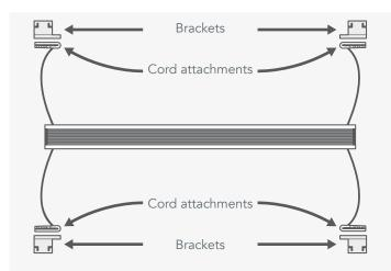
Allocate the brackets so that those with the 'winged' area to the right are used for the left hand side of the blind, and those with the winged area to the left are used for the right hand side of the blind.
